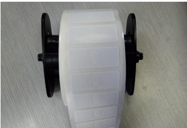
(3) The Media Spindle passes through the label core, pay attention to the direction of the Paper Roll Liner.
