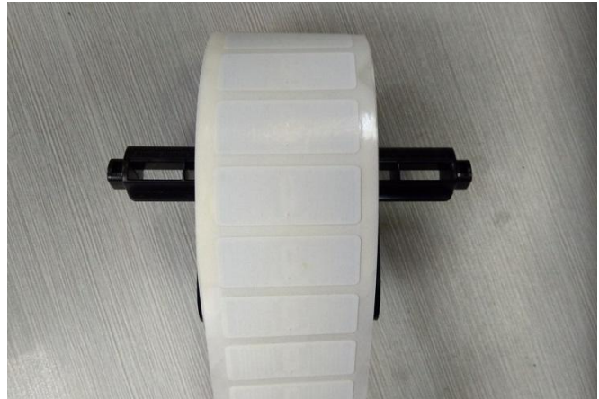
(4) Push in the Media Roll Guide on both sides to center the label, and be careful not to catch it too tightly.
