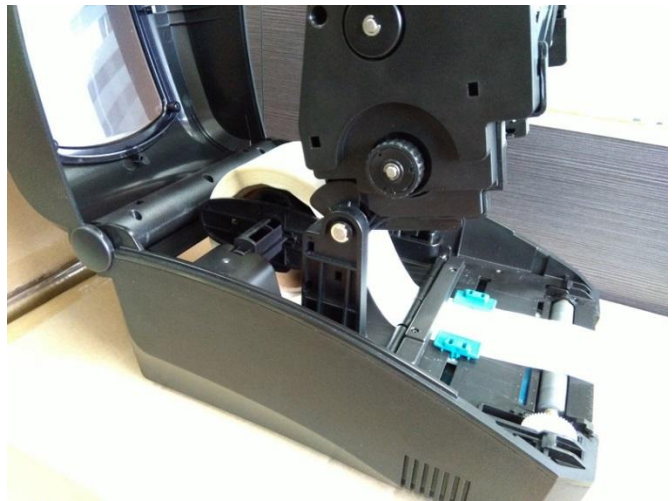
(6) Put the installed paper roll into the paper bin.
